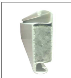
Galvanized steel single skin slats powder coated finish (0.80mm+0.80mm thickness)
